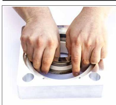
**STEP 5:** With the Faceplate, Shaft wiper & Teflon wear plate removed the wear ring, elastomer & clamp assembly is accessible. Lift the assembly from the housing. Flip the housing and repeat steps 1-4. Rebuild kits include new rings, elastomer and clamp assembly. Take note of how these parts fit together.
