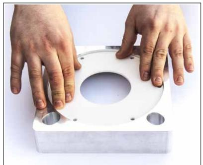
**STEP 7:** Install the Teflon wear ring. Align the holes with the threaded housing faceplate mounting holes.
