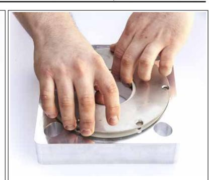
**STEP 2:** With the face plate screws removed you can now remove the outer faceplate. If rebuilding be sure to clean the inside/outside of this plate. Remove any RTV from prior installation. Both faceplates will be reused.
