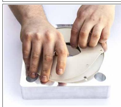
**STEP 3:** Remove the EPDM shaft wiper. If rebuilding a new wiper is included in the kit.
