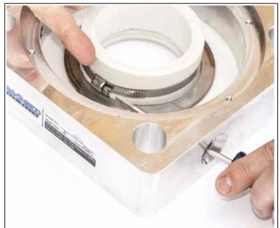
STEP 11: Flip the assembly over. Place a new wear ring polished side down to the Teflon wear plate. Place the elastomer into the wear ring, make sure the screw of the elastomer clamp lines up with the adjustment port as shown.
