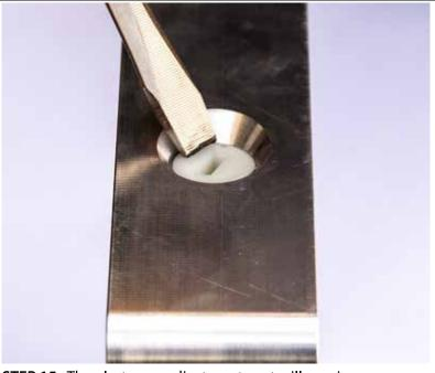
**STEP 15:** The elastomer adjustment port will require reinstallation after the seal has been reinstalled, adjust the elastomer 1/4 to 1/2 turn, snug against the shaft. Do not over tighten the clamp!
