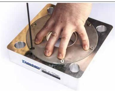
STEP 14: Place the faceplate screws into the mounting holes. With the elastomer/ring assembly inside the seal you will need to apply downward pressure against the faceplate to reinstall it. Use the North/South/East/West method when tightening the screws. Do not over tighten or use thread locker on the mounting screws.
