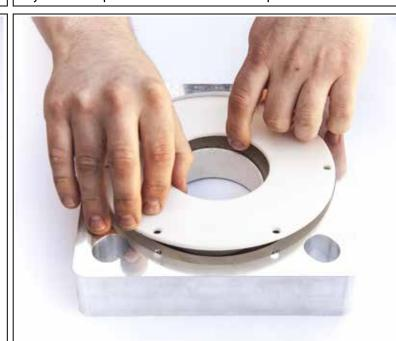
**STEP 4:** Remove the Teflon wear ring.
