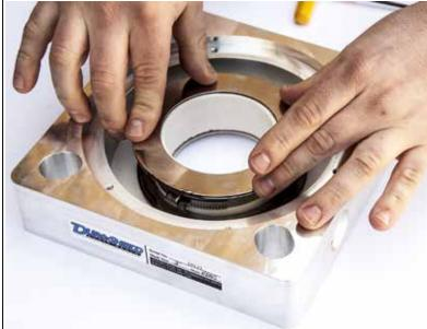
**STEP 12:** Place the remaining Stainless Steel wear ring onto the elastomer. Before proceeding check the fitment of the rings to the elastomer, each ring has a lip and the elastomer fits inside the lip.
