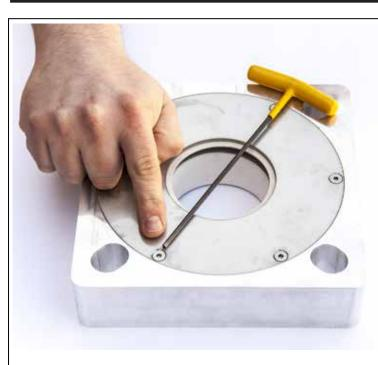
**STEP 1:** Remove the face plate screws using a 1/8" Allen / Hex head wrench. Depending on shaft diameter each seal utilizes a different amount of screws.
