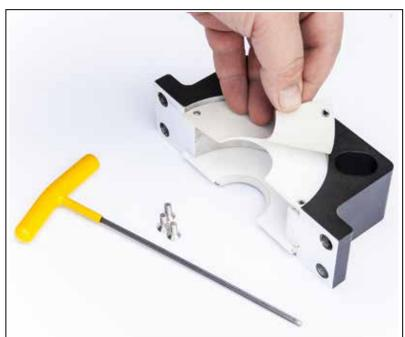
**STEP 5:** Remove the EPDM shaft wiper. The wiper is a thin synthetic rubber material. Rebuild kits include a new set of shaft wipers.
