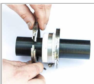
**STEP 18:** The wear rings fasten together using two 7/64" Allen head screws per ring. Insert and tighten the screws adding a 1/4 turn for proper tension. Place the new elastomer & clamp onto the shaft. Seat the elastomer onto the inner lip of the new wear ring. Center the clamp. Install the remaining wear ring.
