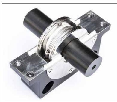
**STEP 19:** When assembled the elastomer/wear ring assembly should fit into the housing. Align the clamp adjustment screw to the adjustment port of the housing- this is crucial for seal adjustment. Verify the clamp is snug but able to move for adjustment.
