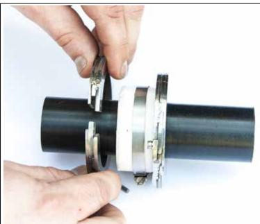
**STEP 16:** With the 7/64" allen screws removed the split ring housings can be removed from the shaft.
