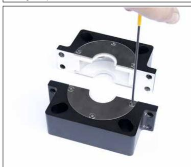
**STEP 3:** With the housing free of the shaft assembly. Remove the faceplate screws using a 1/8" allen wrench.
