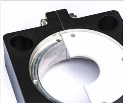
STEP 9: Installing the new wear plates. The wearplates are made in two patterns. Each side of the seal gets one of each pattern. Notice the seam offset created by the larger wearplate. In most seals the wearplates are Teflon. We offer alternate wear plate materials such as Vespel, Peek, Rulon J & Carbon filled teflon. Rebuild kits include a new set of wear plates. Each kit is matched to the seal serial # to assure proper replacement parts.
