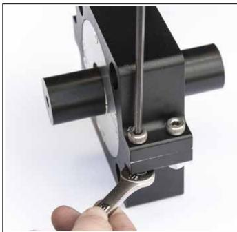
**STEP 1:** Remove the housing shoulder bolts using a 1/2" open/closed wrench & 3/16" Allen wrench. This will allow the seal to seperate into 2 sections. Back the outer faceplate screws out a full turn ,this will allow the two sections of the housing to seperate easier.
