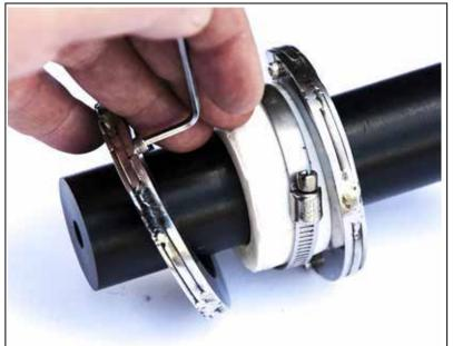
**STEP 15:** The rebuild kit includes new stainless steel rings, elastomer & elastomer clamp. Slide the outer ring forward, using a 7/64" Allen key- Remove the 2 screws which hold the wear ring together.
