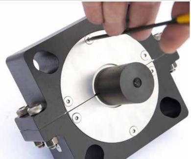
**STEP 22:** Use a 1/8" Allen wrench & tighten the faceplate screws. The faceplates should be flush to the housing. Do not over tighten the screws! An additional 1/4 turn is ample torque.
