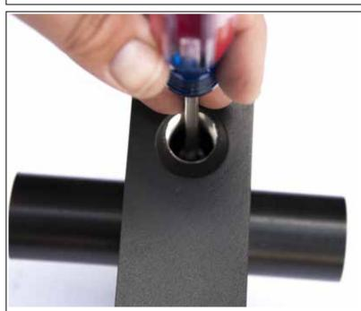
**STEP 23:** With the seal re-installed adjust the elastomer so the shaft rotates normally. Check for rubbing- proper adjustment is crucial for optimal seal life.
