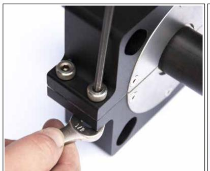
**STEP 21:** Re-install the stainless steel shoulder bolts using the 3/16" Allen wrench & 1/2" open/closed wrench. Fully tighten and apply an additional 1/2 to 3/4 turn. Use of thread locker or anti-seize is not reccomended.
