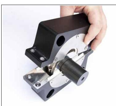
**STEP 2:** With the shoulder bolts removed seperate housing and remove the housing sections from the shaft. NOTE: The black abs shaft is installed to illustrate a typical HDFS installation & how to remove the seal for rebuilding. Internal component disassembly, rebuilding & installation process is illustrated later in this document.
