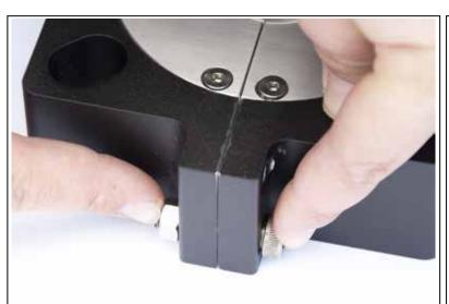
**STEP 13:** Remove the side shoulder bolts and seperate the 2 housing sections.
