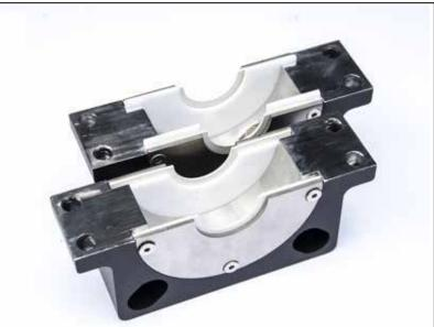
**STEP 14:** Having the faceplate screws backed out a whole turn leaves a small amount of play in the faceplates to allow the seal to reassemble without pinching the internal components. At this stage the housing is rebuilt.
