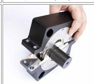
**STEP 20:** Combine the housing segments, Verify the EPDM shaft wipers are not pinched and the Teflon plates are properly seated, the seam should be tight.
