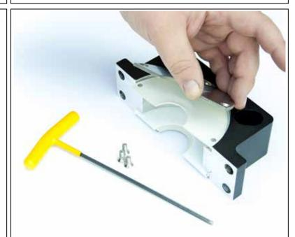
**STEP 4:** Remove the outer stainless steel faceplate
