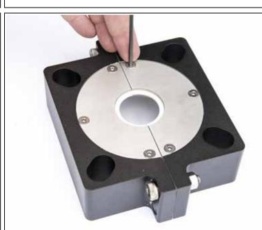
**STEP 8:** Install the faceplates & faceplate screws using the 1/8" Allen wrench. Do not fully tighten the screws as it will not permit the housings to be rejoined properly. Flip the housing and repeat steps 9-8.
