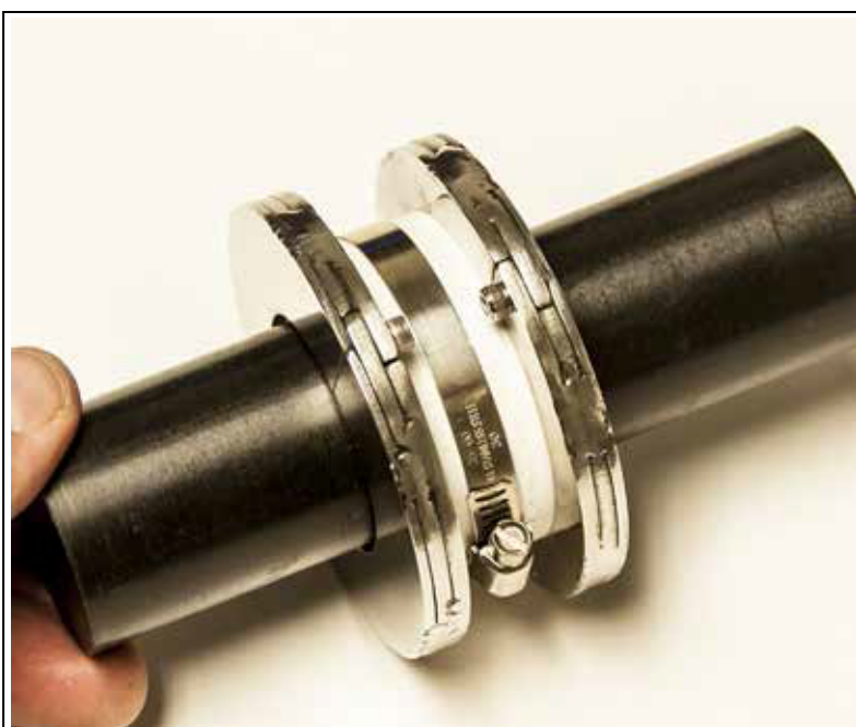
STEP 16: Reinstall the split rings onto the shaft. Make sure the rings properly seat onto the elastomer. The internal assembly should be aligned as shown. Make sure the clamp is centered between the rings.
