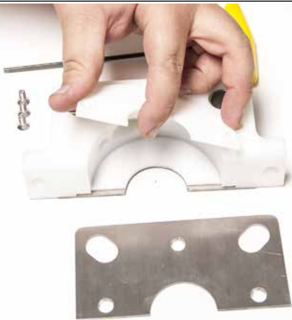
STEP 5: Remove the teflon wear plate. New teflon plates are included with the rebuild kits.
