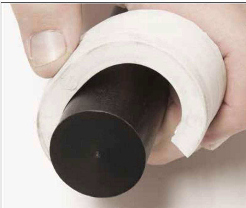
STEP 14: Remove the elastomer clamp, back the clamp screw out using the 3/16" slotted screw driver. the clamp will slip over the elastomer. Remove the elastomer. Rebuild kits include a new EPDM elastomer.
