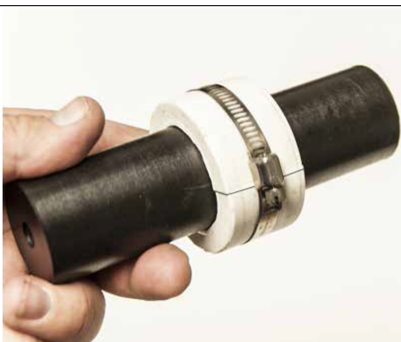
STEP 15: Install the elastomer & elastomer clamp. Align the clamp head over the seam of the elastomer. Form the elastomer gap as tightly as possible by hand before applying pressure to the clamp, tighten the clamp until its seated.
